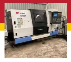
heat dissipation, vibration reduction, and deflection resistance. The machine's compact structure and space-saving design are effective in saving customer space, time and money; while the fully enclosed protection and inclined structure make chip control and continuous chip removal much easier.
